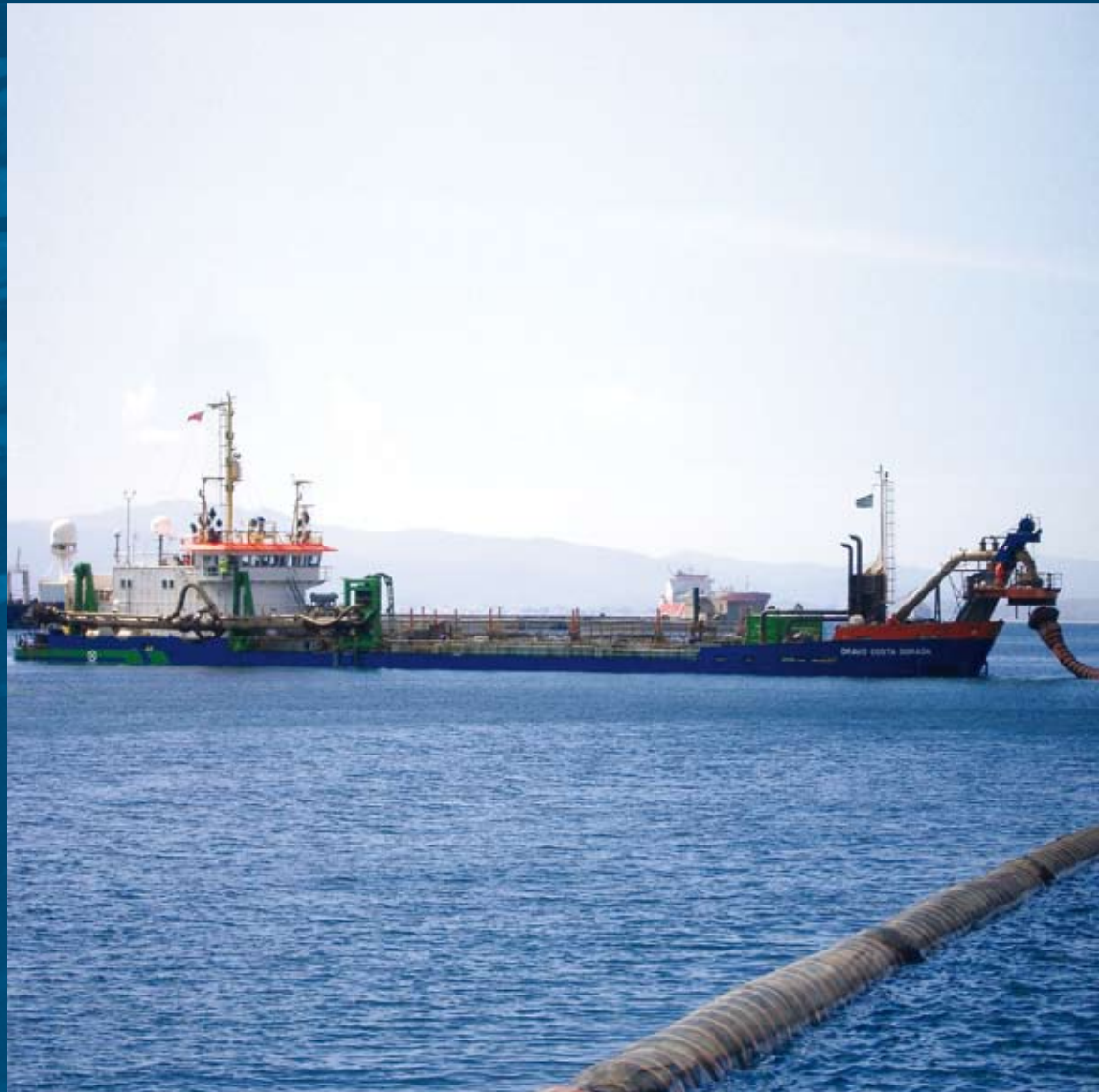
Trailing suction hopper dredger Dravo Costa Dorada
