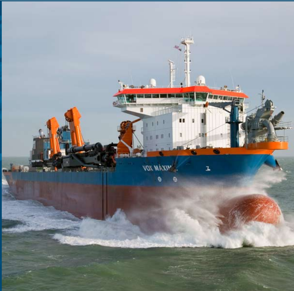
Trailing suction hopper dredger Vox Máxima
