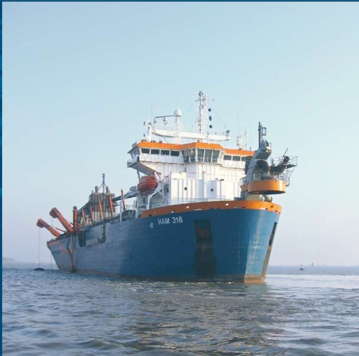
Trailing suction hopper dredger HAM 316
